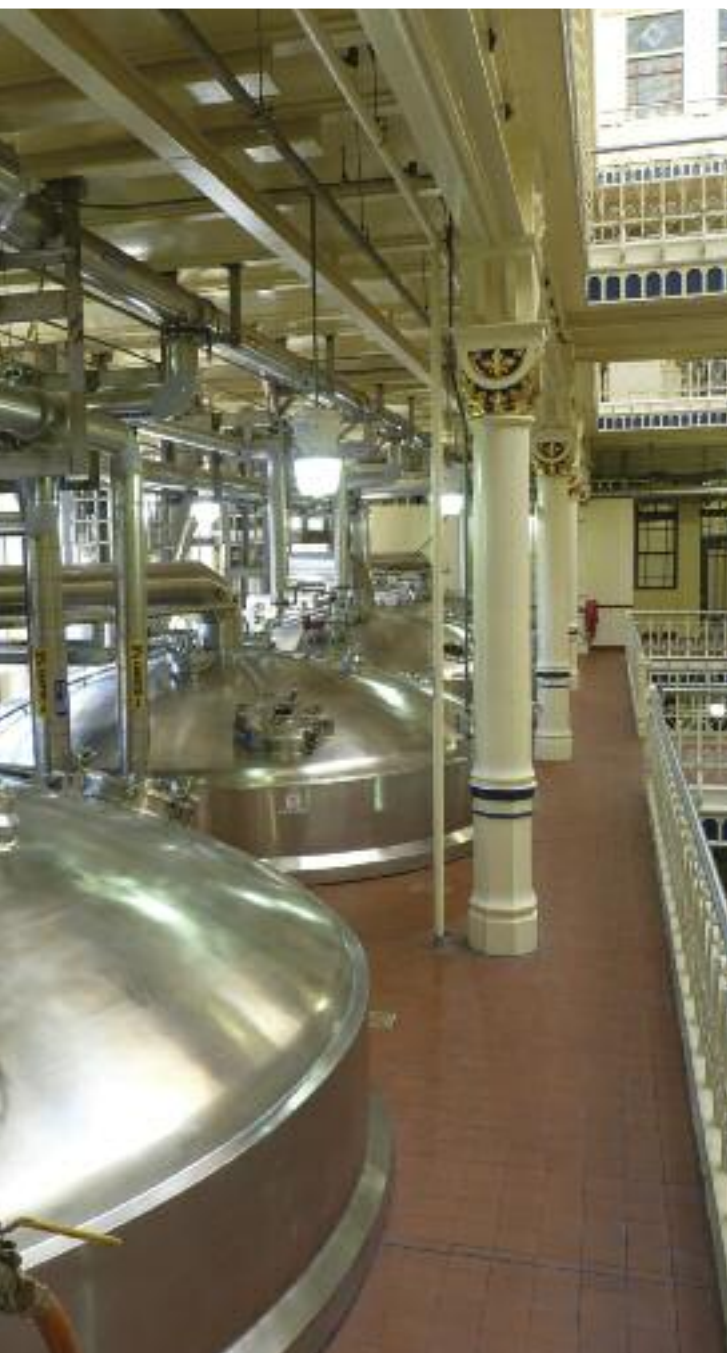
Above: The copper hearth of six vessels and a hoist to raise up the hop bin (inset) which is added to the copper manually.
