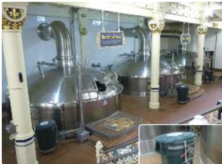
Above: The copper hearth of six vessels and a hoist to raise up the hop bin (inset) which is added to the copper manually.
