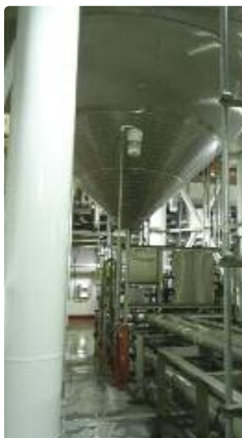
Above: The copper hearth of six vessels and a hoist to raise up the hop bin (inset) which is added to the copper manually.
